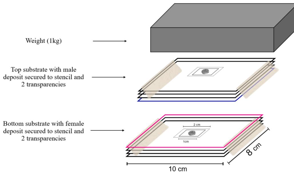
**Fig. 2.** Experimental set up for the friction experiment with female (bottom; pink) and male (top; blue) deposits (not to scale) with substrates affixed together and to the weight with sticky tape.
